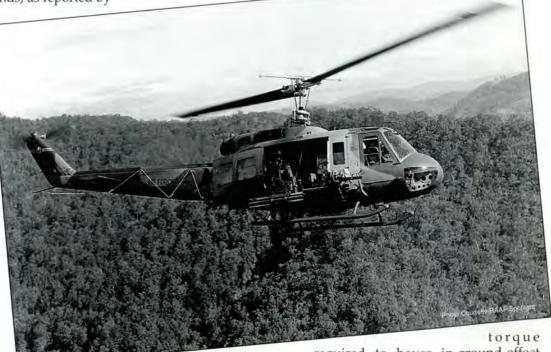
southwesterly wall of the valley. With the combination of at least a 30-knot quartering tailwind, a planned descent, entering a downdraft condition, and an initiated right turn, the rate of descent increased so rapidly the pilot was unable to keep the aircraft from crashing.
